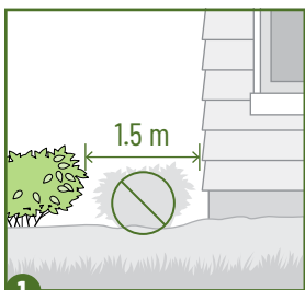
1 Remove all combustible ground cover (mulch and plants) within 1.5 m of the house perimeter.
